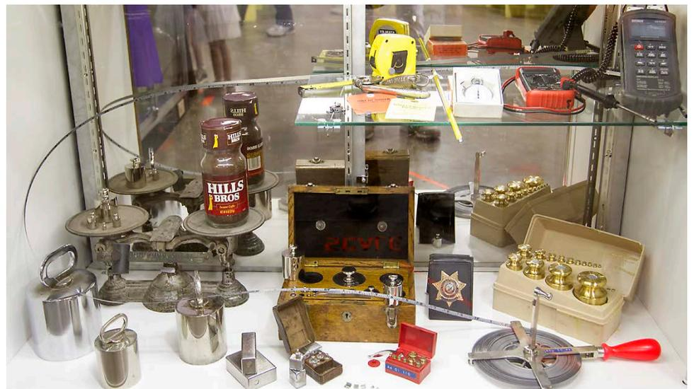
*Various tools used by Weights and Measures inspectors to test the accuracy of weighing and measuring devices in the market place.*
